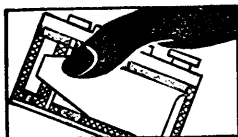
Insert film spool on take-up side, insert roll-film, fix paper end.
